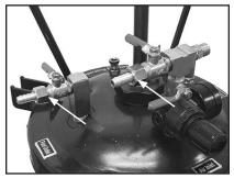
Figure 4. Spray gun fittings installed.
